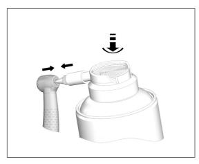
Lubrication of the chucking system
